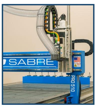
much cutting you perform you will not get failure to the bearings. The design also makes the machine a self-cleaning system without the worry of wiping down the rails or watching for buildup.
